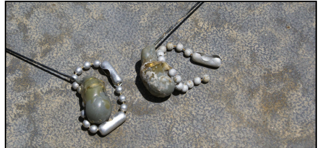
FIGURE 3. Holohil BD2 radio transmitters originally attached to Blunt-nosed Leopard Lizards ( Gambelia sila ) at study sites in Kern County, California. The transmitter on the left was removed from a living lizard and the transmitter on the right was found in the tunnel of a kangaroo rat ( Dipodomys sp.). Note the dulled surface of the beaded chain collar and the discoloration of the transmitter on the right. This transmitter likely passed through the digestive system of an animal, probably a snake. (Photographed by David J. Germano).
